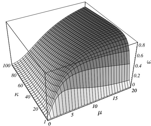
Figure 17: Convergence  $\omega$  of Steepest Descent as a function of  $\mu$  (the slope of  $e_{(i)}$ ) and  $\kappa$  (the condition number of  $A$ ). Convergence is fast when  $\mu$  or  $\kappa$  are small. For a fixed matrix, convergence is worst when  $\mu = \pm\kappa$ .
