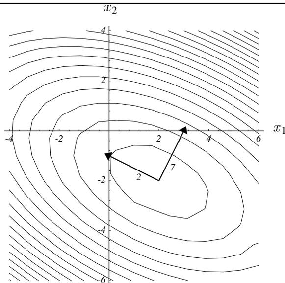
Figure 12: The eigenvectors of  $A$  are directed along the axes of the paraboloid defined by the quadratic form  $f(x)$ . Each eigenvector is labeled with its associated eigenvalue. Each eigenvalue is proportional to the steepness of the corresponding slope.
