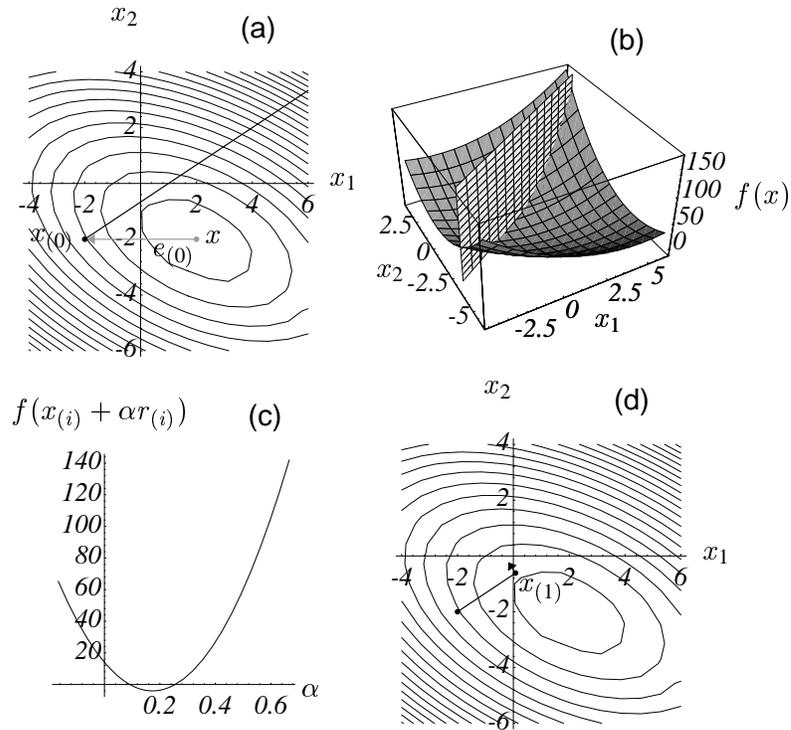
Figure 6: The method of Steepest Descent. (a) Starting at  $[-2, -2]^T$ , take a step in the direction of steepest descent of  $f$ . (b) Find the point on the intersection of these two surfaces that minimizes  $f$ . (c) This parabola is the intersection of surfaces. The bottommost point is our target. (d) The gradient at the bottommost point is orthogonal to the gradient of the previous step.
