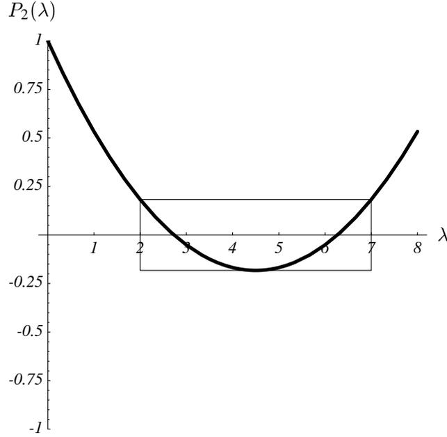
Figure 33: The polynomial  $P_2(\lambda)$  that minimizes Equation 50 for  $\lambda_{min} = 2$  and  $\lambda_{max} = 7$  in the general case. This curve is a scaled version of the Chebyshev polynomial of degree 2. The energy norm of the error term after two iterations is no greater than 0.183 times its initial value. Compare with Figure 31(c), where it is known that there are only two eigenvalues.
