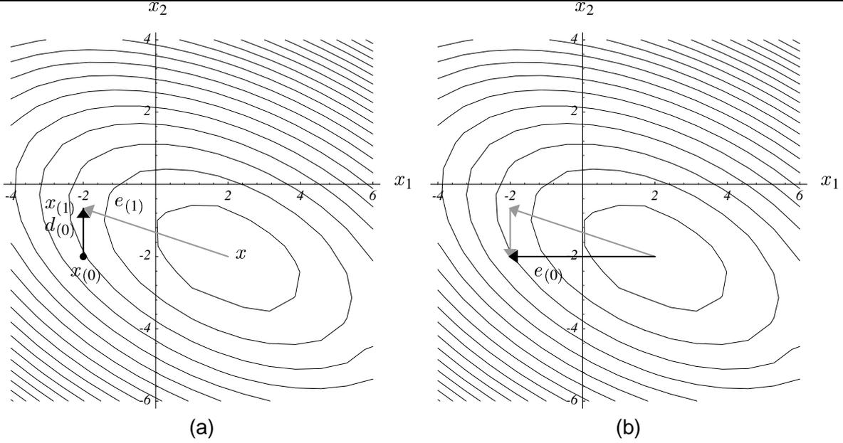
Figure 23: The method of Conjugate Directions converges in  $n$  steps. (a) The first step is taken along some direction  $d_{(0)}$ . The minimum point  $x_{(1)}$  is chosen by the constraint that  $e_{(1)}$  must be  $A$ -orthogonal to  $d_{(0)}$ . (b) The initial error  $e_{(0)}$  can be expressed as a sum of  $A$ -orthogonal components (gray arrows). Each step of Conjugate Directions eliminates one of these components.
