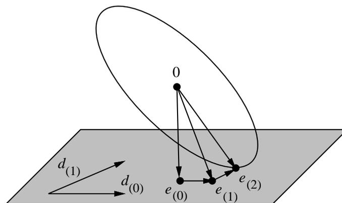
Figure 26: In this figure, the shaded area is  $e_{(0)} + \mathcal{D}_2 = e_{(0)} + \text{span}\{d_{(0)}, d_{(1)}\}$ . The ellipsoid is a contour on which the energy norm is constant. After two steps, Conjugate Directions finds  $e_{(2)}$ , the point on  $e_{(0)} + \mathcal{D}_2$  that minimizes  $\|e\|_A$ .
