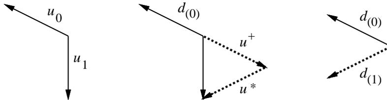
Figure 24: Gram-Schmidt conjugation of two vectors. Begin with two linearly independent vectors  $u_0$  and  $u_1$ . Set  $d_{(0)} = u_0$ . The vector  $u_1$  is composed of two components:  $u^*$ , which is  $A$ -orthogonal (or conjugate) to  $d_{(0)}$ , and  $u^+$ , which is parallel to  $d_{(0)}$ . After conjugation, only the  $A$ -orthogonal portion remains, and  $d_{(1)} = u^*$ .
