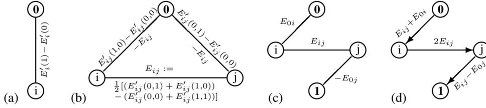
Figure 1: Equivalent Ising model (with disagreement costs) for a given (a) node energy  $E'_i$ , (b) edge energy  $E'_{ij}$  in a binary graphical model; (c) equivalent submodular model if  $E_{ij} > 0$  and  $E_{0i} > 0$  but  $E_{0j} < 0$ ; (d) equivalent directed model of Kolmogorov and Zabih [1], Fig. 2d.
